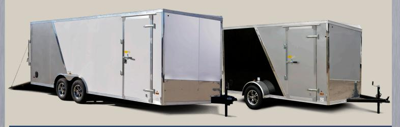
SUPER LOCK... Exterior Aluminum system is unique to Haulin Lasts longer, looks much better, resists rust much better. The interlocking aluminum panels are glued and mechanically fastened so that it is not exposed to view or the weather.
