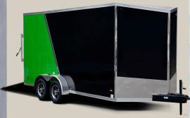
Six wide models and up have a double rear door standard. 5 wides come with single door due to size limitation. Ramp door optional upgrade is available. All doors have advanced automotive door seals to lock out dust, moisture, and road grime for superior protection.
